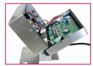
Internal Hinge Mechanism Easy access for option installation and servicing
